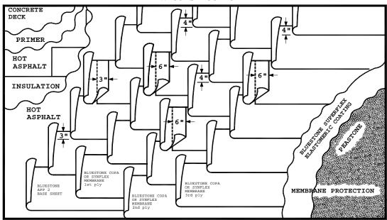
The top ply must have lap in center of the underlying ply.
