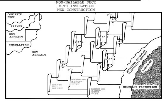
The top ply must have lap in center of the underlying ply.
