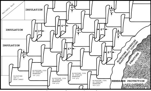
The top ply must have lap in the center of the underlying ply.
