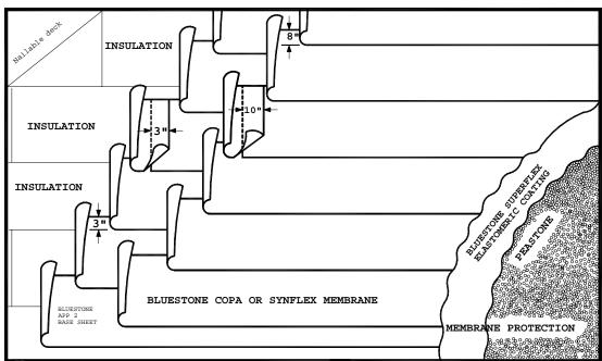
The Bluestone membrane should have lap in the center of the base sheet.
