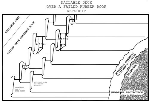
The top ply should have lap in the center of the base sheet.
