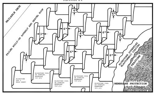
The top ply must have lap in center of the underlying ply.
